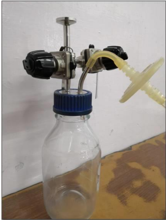
Design of sampling assembly with collection bottle
